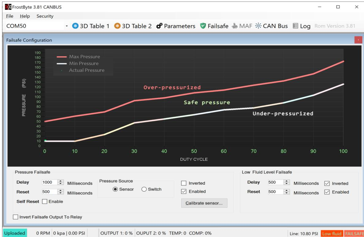
In the photo above you will notice that there are two pressure profiles traced by red and white lines. Users will set their pressure profiles based on what the device does in previous logs. The lines can be clicked-dragged to form the correct safe pressure boundary.
